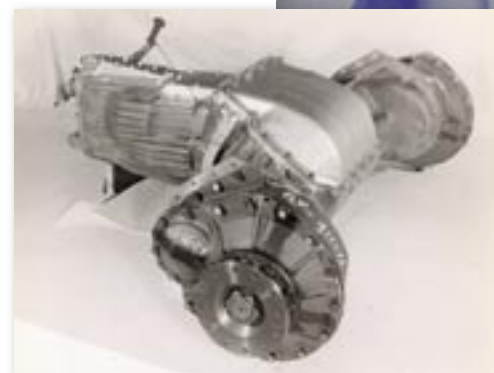
Spicer products were used on a wide variety of military vehicles. Pictured here is a Spicer transmission for a Landing Vehicle Tracked (LVT) "Water Buffalo" used by the U.S. Marines.
