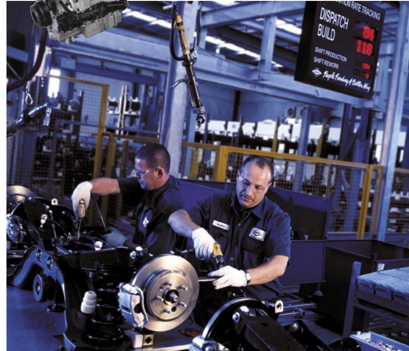
Matthew Kelly (left) and Vlado Kova assembled suspension modules for the Ford Falcon car in Dana's Campbellfield, Australia,
