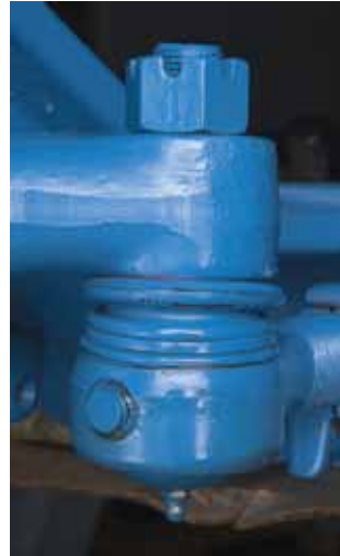
Patented purge valve tie rod end with sealed boot.
