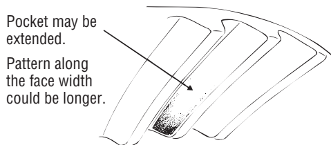
Correct Pattern Used Gearing
