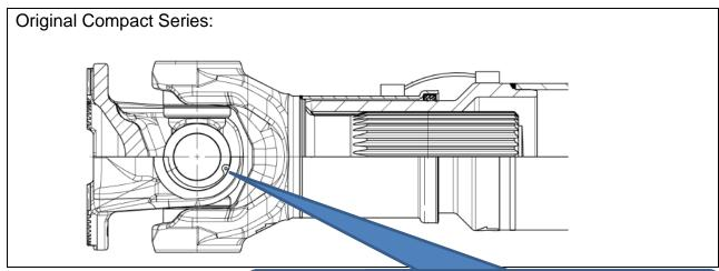
The replacement U/J kits, Flange yokes and Center bearings are interchangeable from **Original** to the **New/Current**.
